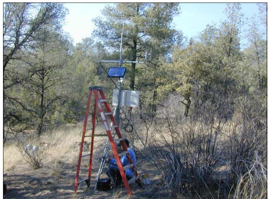
ET/climate station near completion as Stan Engle, NM Climate Center, attaches instrumentation to solar panel and battery. April 2008.
