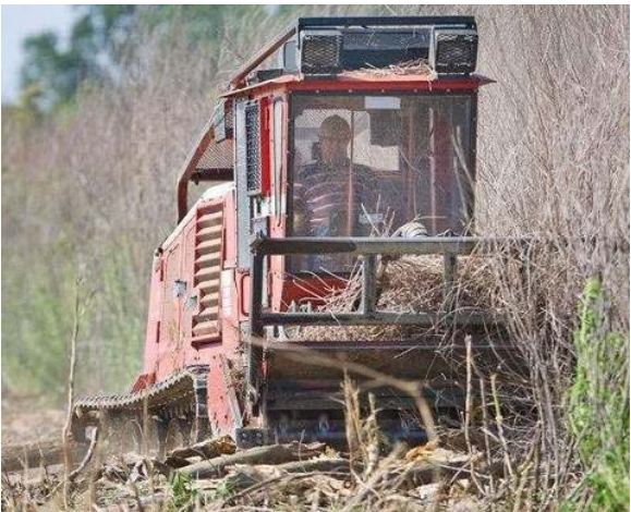
A KMC 1100 Hydrostatic Mulcher, with Ben Bowman of Ballinger, Texas, in the driver's seat, chews up stands of reeds and trees 10 to 15 feet tall with its 48 teeth. It can cut an 8-foot swath. The foliage was sprayed with an herbicide last year so that it could be removed. ALYSSA SCHUKAR/THE WORLD-HERALD
